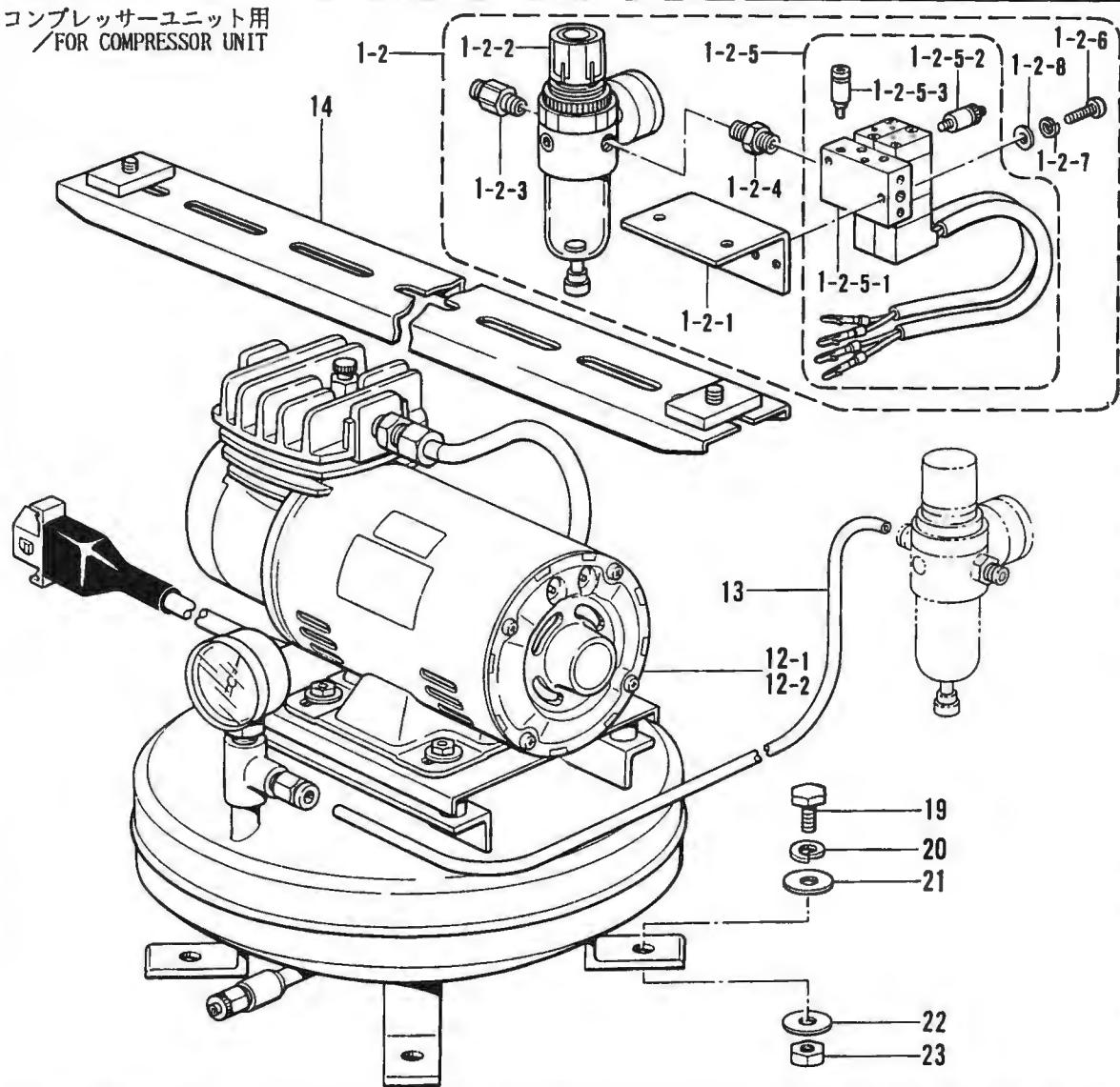
R. 空圧関係/Air pressure mechanism/Luftdruck/
